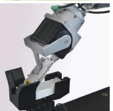
Fixed finger: it allows to mount different equipments for special purposes. Precise, strong, and at the same time adaptable thanks to Variable Stiffness<sup>TM</sup>.
